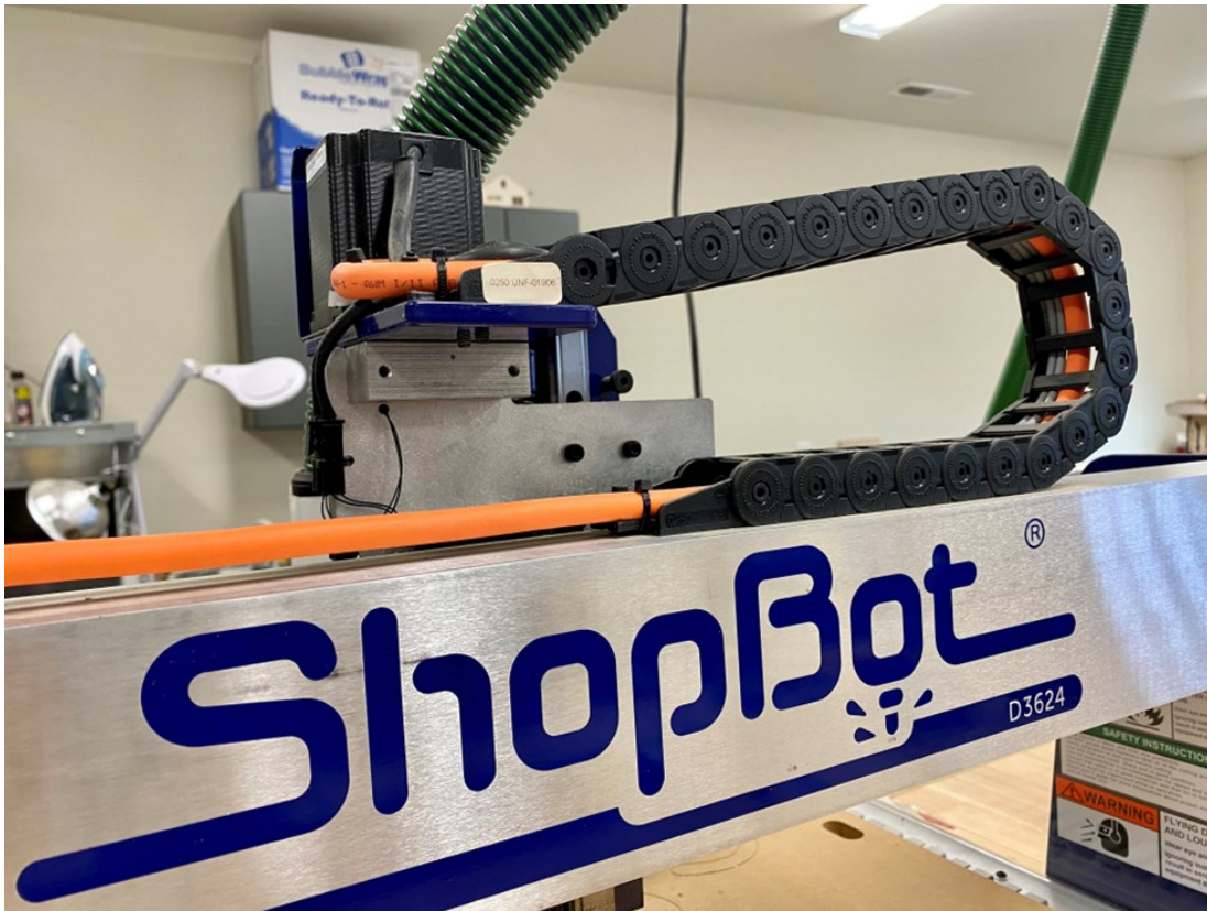
36" x 24", Bosch 1hp high-speed-spindle, 3-axis CNC machine
