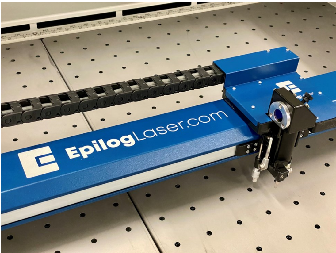
80 watt, 48"x36", 1200dpi etch, 1/2" hardwood cut, auto-focus, vacuum table, remote video monitor, full registration 2-sided capable laser from Epilog
