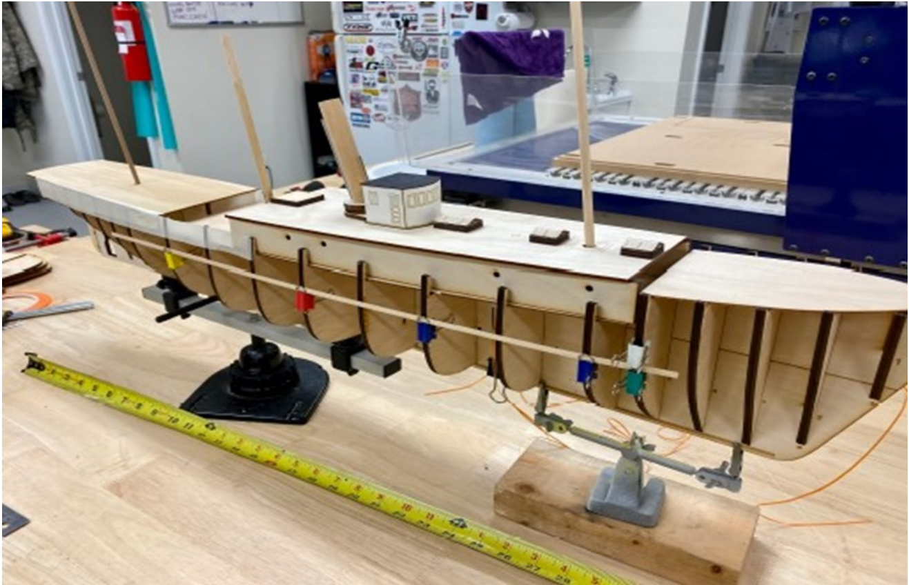
US Revenue Cutter Bear prototype in 1:64. Designed from Smithsonian drawings
